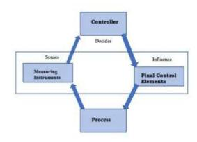
Block diagram of basic Instrumentation Control system
